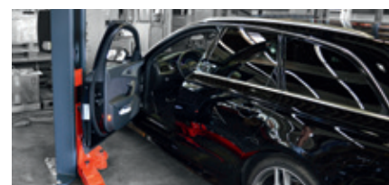
Large door opening angle, door stop protection
