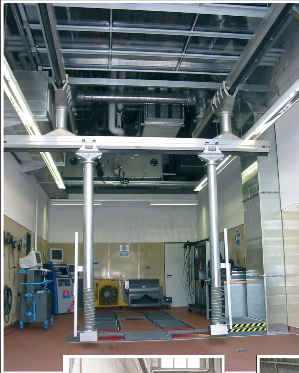
Rail system SSK 290 as movable coordinate system for passenger car performance test beds with suction performance of up to 4,000 m 3 /h and available as high temperature version for exhaust gas temperatures of up to 900°C.
