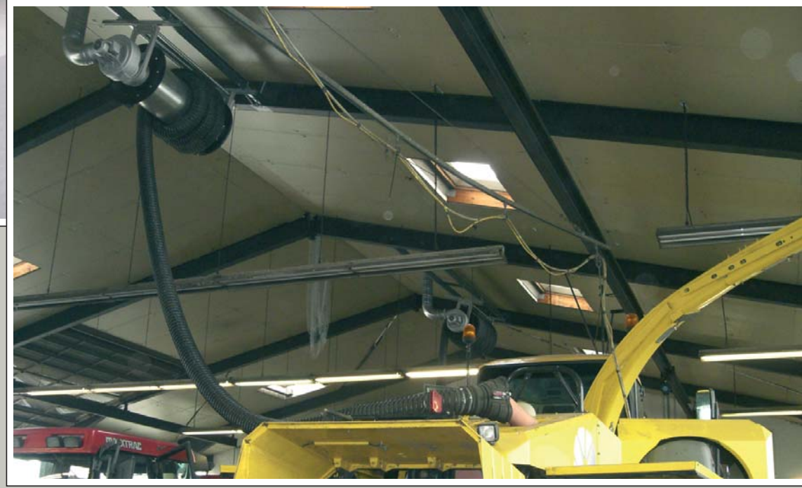
Hose reel with aluminium casing and motor drive for agricultural machine workshops.
