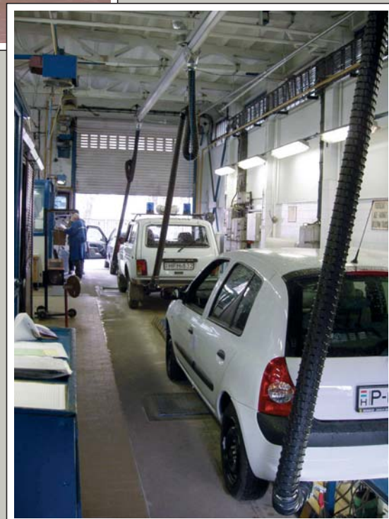
Rail system SSK 290 as round trip carrier system for technical vehicle control inspection boards with a high vehicle frequency of up to 150 vehicles per test track.
